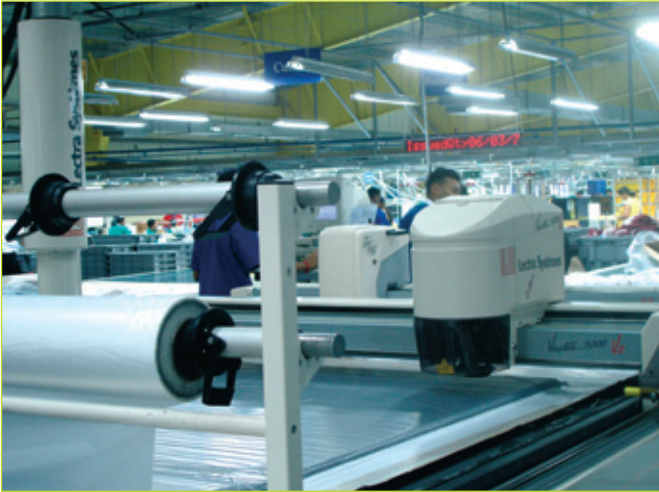
Linea Aqua uses three Lectra Vector 5000 V2 computerised cutters as shown above.
