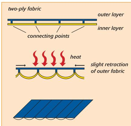
**Kermel's R-Liner reactive process creates tubular channels as an air barrier.**
