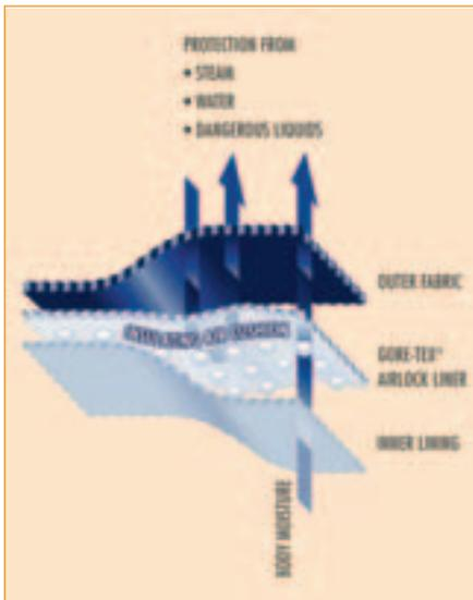
**Gore-Tex Airlock - designed to operate under the most hazardous conditions.**
