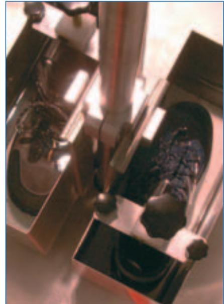
*Extensive waterproof testing at Gore laboratories includes the Mechanical Boot Flex Tester (left) and the Centrifugal Tester (right).*
