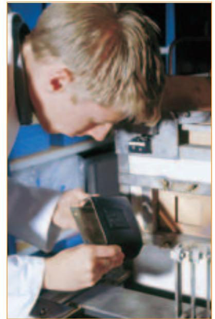
**Contact and Radiant heat testing.**
