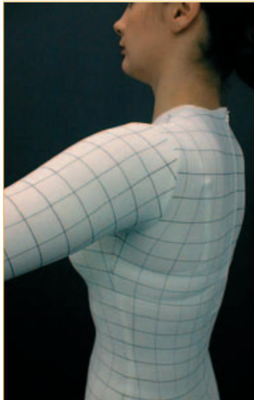
*A 25mm grid system printed on the analysis body suit is an important aid in evaluating stretch-fit.*
