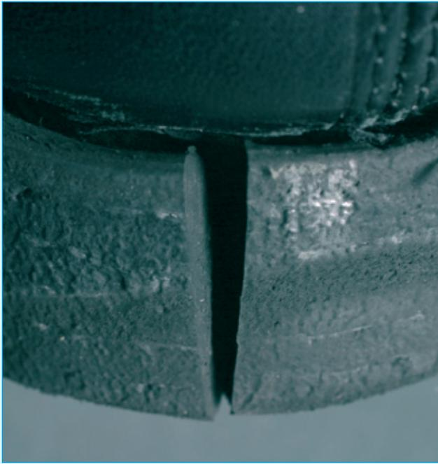
*This heel has split, probably at the mould flow line, due to the realistic compression applied by the tester.*
