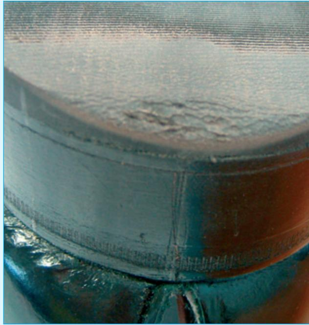
*The wear pattern at the rear of a rubber top piece after the machine test.*
