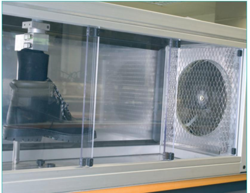
*The SATRA test comprises a heated foot form suspended in a wind tunnel.*
