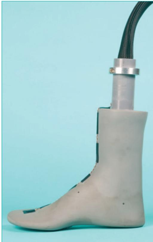
Foot form with hose attached prior to testing
