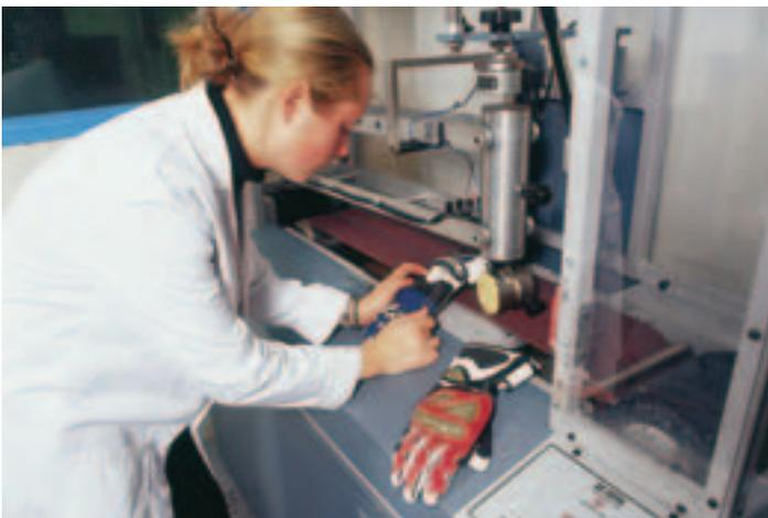
*Motorcycle glove abrasion is tested by a test specimen being dropped from a height of 50mm onto an abrasive belt. The belt moving at a speed of 8 m/s produces a contact force of 49N. The time to abrade through the full thickness of the sample is then measured by an electronic timer triggered by a system of trip wires.*
