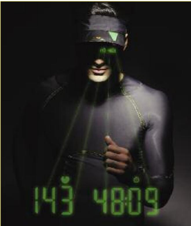
*The Screeneye X visor, developed by German company O-Synce, is mounted with a digital display to project data directly to the user's field of vision. The device is powered by a UV-light harvesting film placed on top of the visor or charged via USB.*
