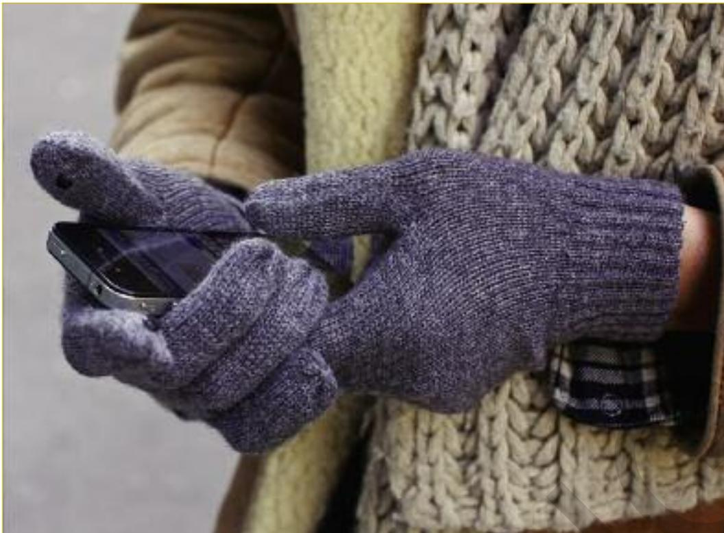
*Glovetip, designed by French start-up Chi&Jo, is based on a pine-tree shaped tip that attaches to any glove to use smart tactile devices in cold weather. A combination of a conductive plastic with a stainless steel tip activates tactile screens, which are no longer resistive (or pressure-based), but use static electricity emitted by the skin.*
