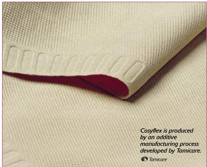
*Cosyflex is produced by an additive manufacturing process developed by Tamicare.*
