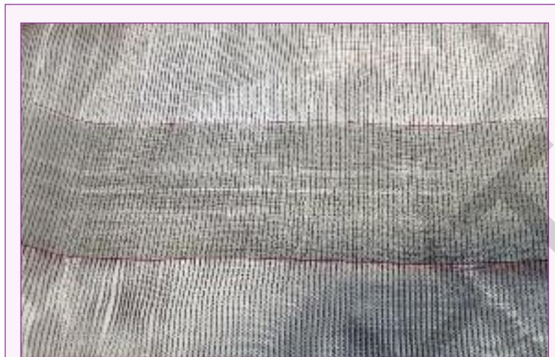
*This c fabric, presented at Itma in 2015, can generate (10W/m<sup>2</sup>) and store (10Wh/m<sup>2</sup>) energy in a fully textile matrix. It combines photovoltaic fibres, based on perovskite solar cells, and rechargeable energy-storing fibres containing a thin battery film.*
