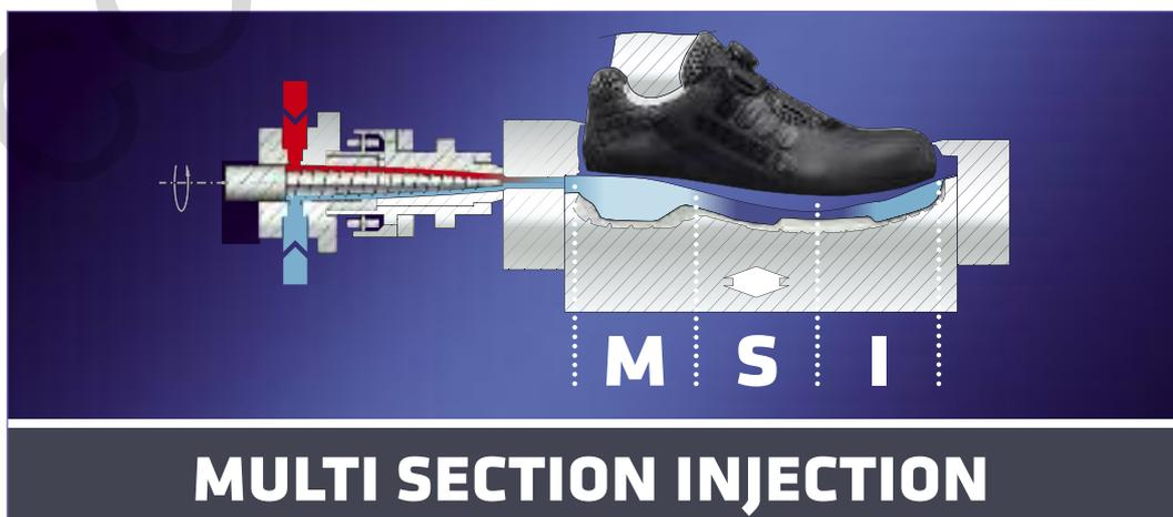
*Desma’s MSI machinery allows for custom mixing of PU components in the chamber.*
