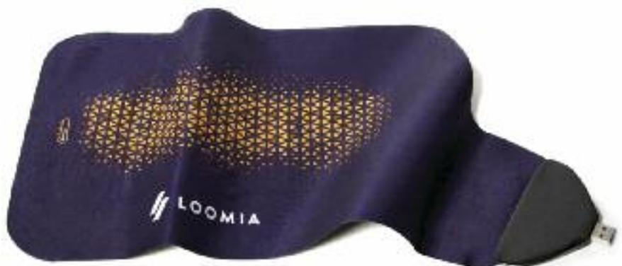
Massachusetts, introduced a new offering allowing the application of printed electronic circuits on what the company calls “washable textiles”. These are said to be able to withstand 50 machine-wash and heated dryer cycles. The company also claims that they enable direct printing onto synthetic fabrics, including polyester, spandex and nylon, with “no need for dielectric encapsulation to ensure wash durability”.
