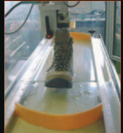
prevent slipping. The initial slipping movement must be contained (static rubbing) and the speed of the slide must be limited so as not to lose balance (dynamic rubbing). Within the framework of European standards on slip-resistance for professional footwear (NF EN 13287), CTC has developed testing equipment that has since been used to test urban footwear.
